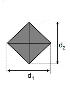
Hardness is defined as the pressure on the contact area of the indentation impression: For the 'Vickers' diamond pyramid profile the Vickers Hardness Number (HV or VHN) is given by:
