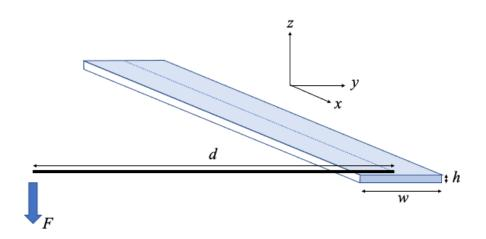
The shear stress  $\tau$  (or  $\sigma_{xy}$ ) at the beam surface along the dotted line is given by
