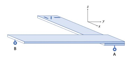
Figure 1: The cantilever beam with strain gauges, used for bending and torsion experiments
