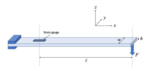
Due to the applied force *F*, a couple of moment  $F\ell$  (the bending moment) acts on the beam cross section at the gauge position.
