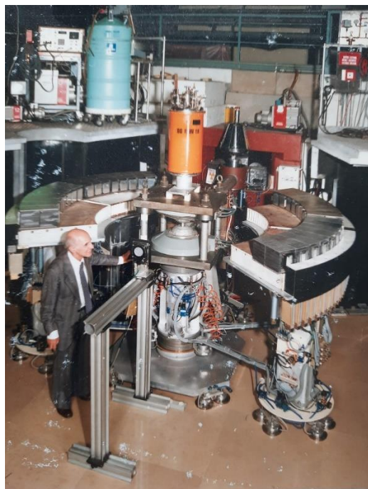
Figure 1 D7 instrument showing an array of detectors enveloping the central part with an orange cryostat in situ. For detailed description see Fig. 3.1, p. 31 in the main text.
