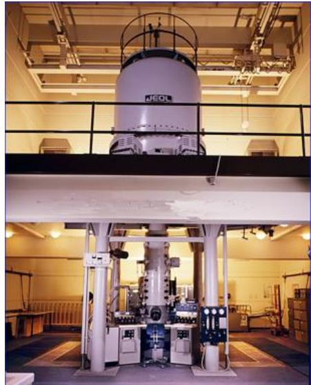
To appreciate the scale of this microscope, here is a closer look at the lower section. The microscope spans three floors; the basement with the pneumatic dampening system is not shown in either photo.
