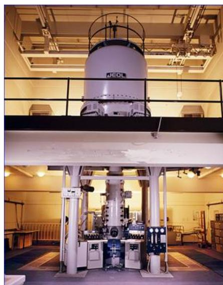
To appreciate the scale of this microscope, here is a closer look at the lower section. The microscope spans three floors; the basement with the pneumatic dampening system is not shown in either photo.
