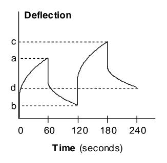
Measured results of pulsed load
