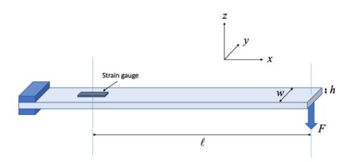
Due to the applied force F, a couple of moment  $F\ell$  (the bending moment) acts on the beam cross section at the gauge position.
