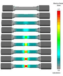
Figure 3. Tensile test necking simulation
